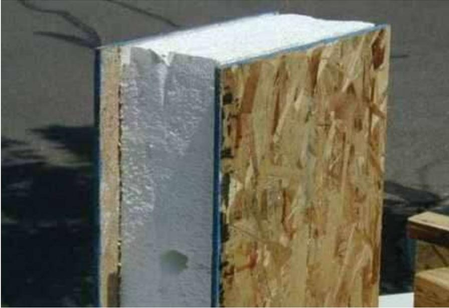
Fig 4: Structural Insulated Panel (SIP)
