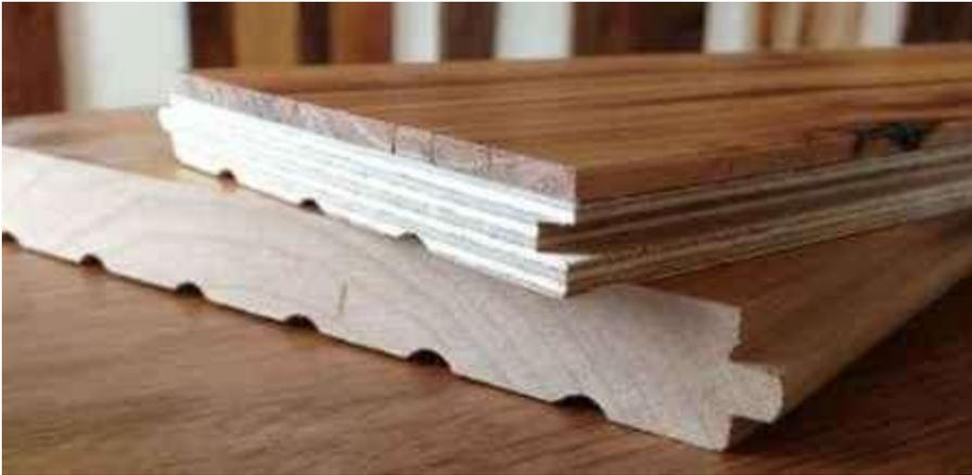
Fig 2: Engineered Wood Board over Solid Wood Board
