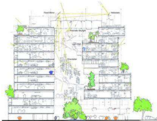
FIG. 2.9 Conceptual section of Genzyme Corporation at Cambridge, USA showing the surplus natural energy inside the building.
