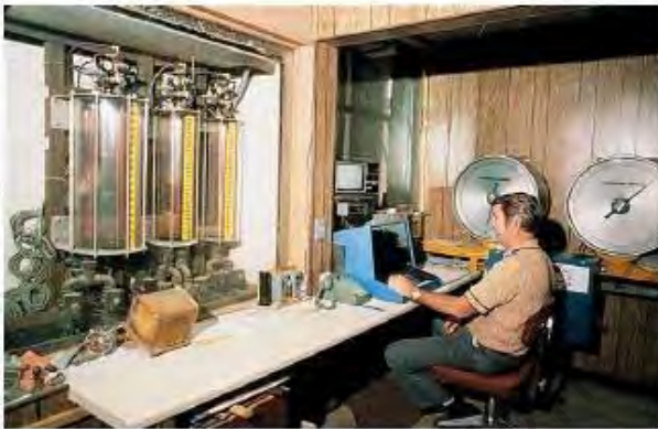
Liquid admixture dispenser at a ready mix plant provides accurate volumetric measurement of admixtures.
